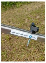
Insert ¼ " bolt through ARM slot and replace washer.
