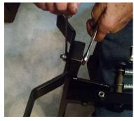
Tighten lock nut very tightly with wrenches.
