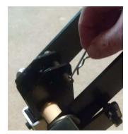
Remove the CLEVIS PIN from bottom of the ARM.
