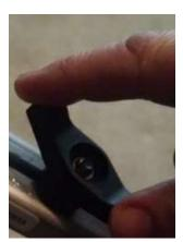
Screw on the Plastic Wing Nut and tighten by hand.
