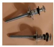
Place Carriage bolt head in slot on the Front Leg. A washer, lock washer and nut are used to lock it in place. Use 9/16" wrench to tighten both spikes FIRMLY.
